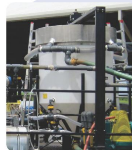
STEP 3 - Chemical separation using Ferric Sulfate to remove fine particles
